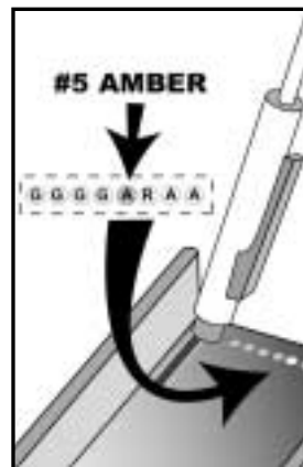
Figure 11 - Magnetic reed switch / LED location.
