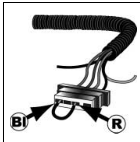
Figure 32 - Full field jump wire.
