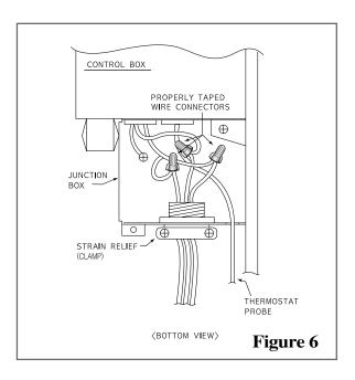
IF INSULATED CABLE IS NOT AVAILABLE, APPROPRIATE STRAIN RELIEF CONNECTORS OR CLAMPS SHOULD BE USED.
